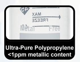
TotalPure™ Centrifuge Tubes are made with a proprietary purified polypropylene blend that reduces the metallic content present in most plastic blends to less than 1ppm. They also feature an array of premium performance and visual features.
